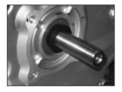
4. Screw the supplied 7/16-14 hex head cap screw into the impeller snout. As the bolt is tightened the impeller will be pried off of the shaft of the drive unit. Remove the 7/16-14 screw once the impeller has been removed from the drive unit.
