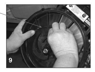
10. Install the volute (12702A) onto the rear bracket using the three volute screws (1-(12900), 20(12725)). Install the check valve (12705) onto the snout of the volute. The drive unit should be turned over a few times to check for clearance between the impeller and volute. A small amount of drag between the impeller and volute will cause no problem, however, if the drive unit will not turn over because of the lack of clearance a bracket shim may have to be used.
