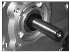
3. To install the carbon seal half into the rear bracket use a tool such as a 1 ½" pipe nipple or arbor press to give even pressure on the metal flange of the seal housing during installation.
